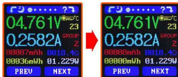
With a Data Group selected, press and hold the 'PREV' button to clear the mAh and mWh. (As shown)
