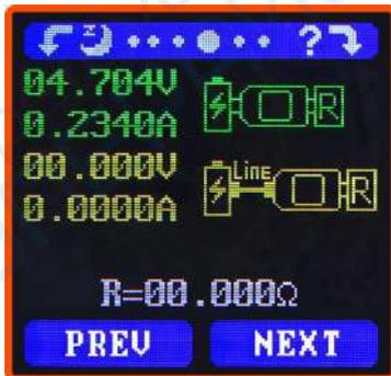
Data Connection Cable Impedance Measurement Interface
