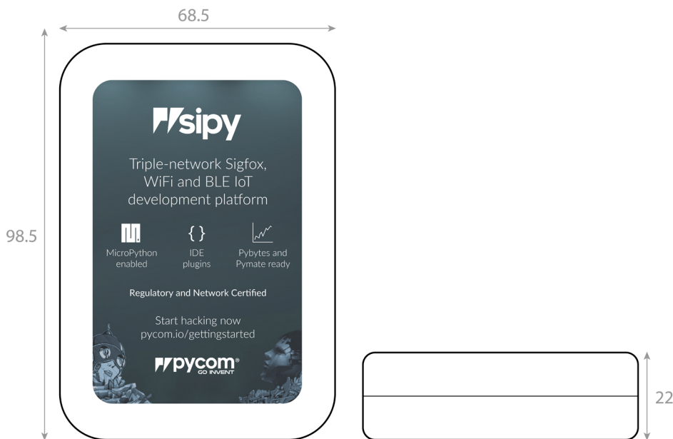
Figure 10 – Mechanical drawing of packaging – Units: mm
