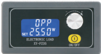
Set over power protection (OPP) Default 35.5W
