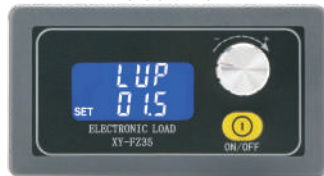
Set low voltage protection (LVP) Default 1.5V
