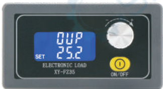
Set over power protection (OPP) Default 35.5W
