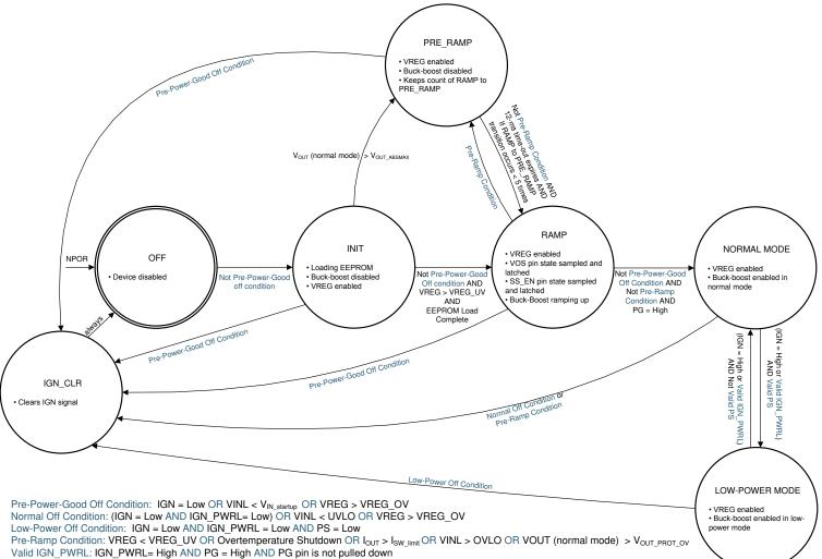
Valid IGN\_PWRL: IGN\_PWRL= High AND PG = High AND PG pin is not | Valid PS: PS = High AND PG = High AND PG pin is not pulled down
