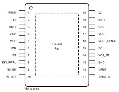
Figure 6-1. PWP PowerPAD<sup>™</sup> Package 20-Pin HTSSOP With Exposed Thermal Pad Top View
