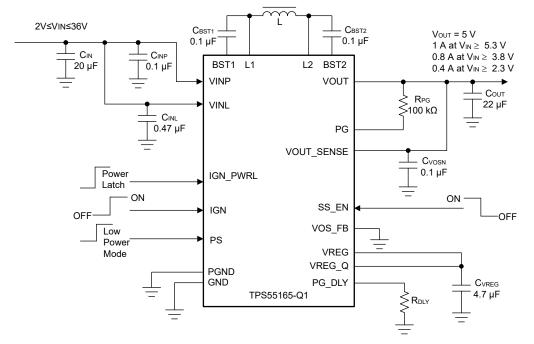
Figure 9-5. TPS55165-Q1 Buck-Boost Converter for Fixed 5-V Output
