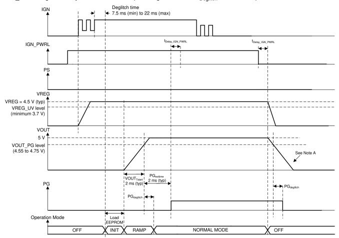
A. The actual ramp-down time of the output voltage depends on external load conditions.
