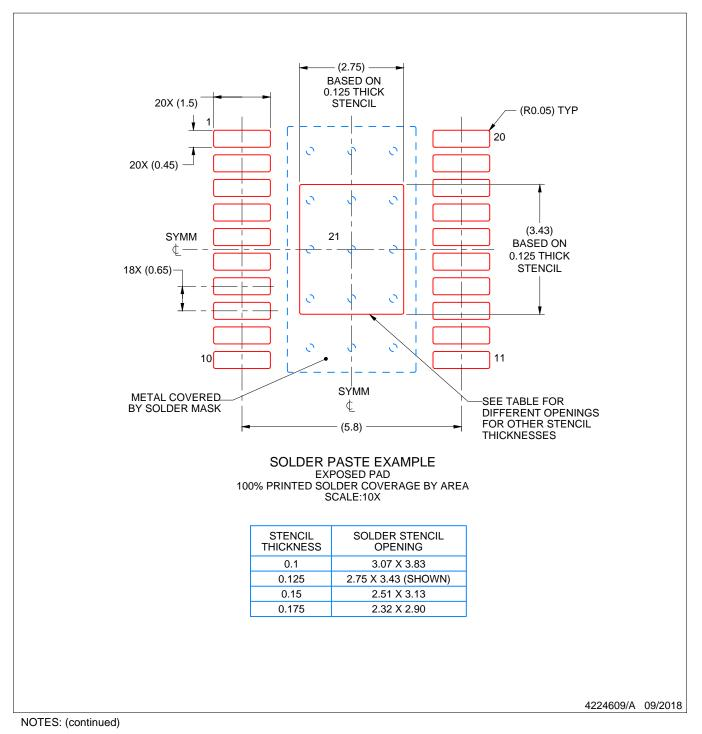
Laser cutting apertures with trapezoidal walls and rounded corners may offer better paste release. IPC-7525 may have alternate design recommendations.
