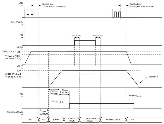
A. The actual ramp-down time of the output voltage depends on external load conditions.
