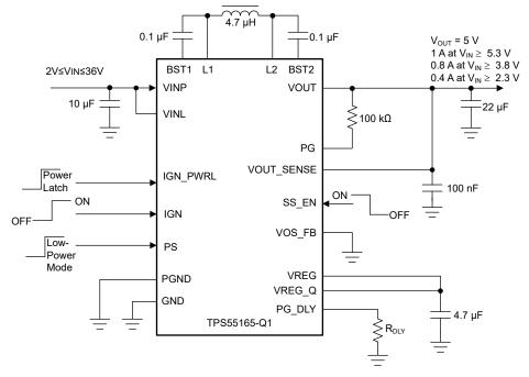
Figure 9-3. TPS55165-Q1 Application Diagram for 5-V Voltage
