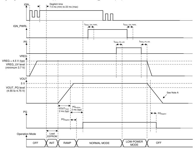
A. The actual ramp-down time of the output voltage depends on external load conditions.
