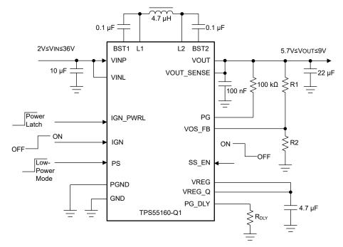
Figure 9-1. TPS55160-Q1 Application Diagram for Adjustable Output Voltage
