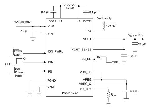
Figure 9-4. TPS55165-Q1 Application Diagram for 12-V Voltage
