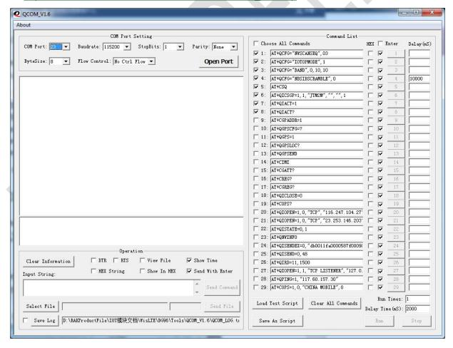
Send AT, the device returns OK to prove that the device is normal, detailed AT commands refer to BG96's AT manual.
