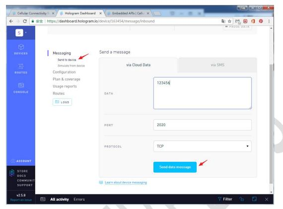
After the Hologram Dashboard is sent, the device will receive a message of "recv, 11" indicating that the device received the data. At this time, the AT+QIRD=11,1500 command is sent to obtain the received data.
