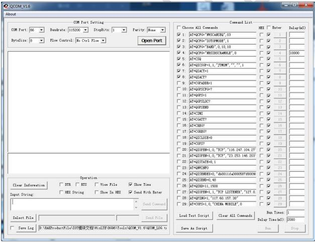
Serial port settings see below ,Send AT, the device returns OK to prove that the device is normal, detailed AT commands refer to BG96's AT manual.
