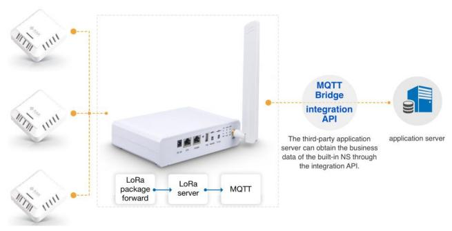
Figure 1 | Typical deployment scenario
