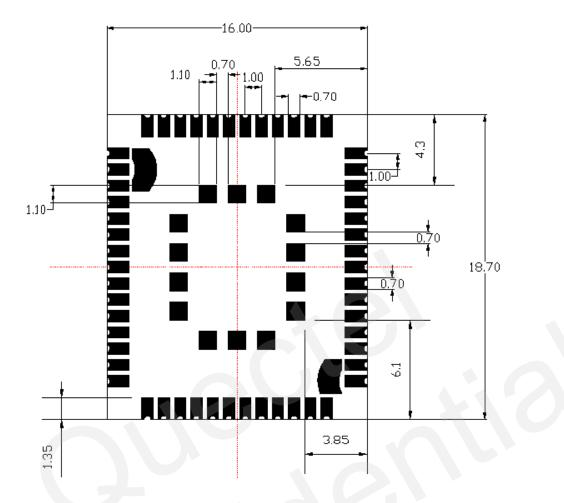
Figure 43: MC20 Bottom Dimensions (Unit: mm)
