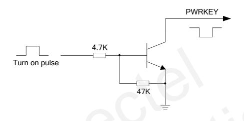
Figure 11: Turn on the Module with an Open-collector Driver
