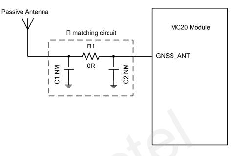
Figure 40: Reference Design with Passive Antenna
