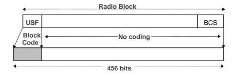
Figure 51: Radio Block Structure of CS-4
