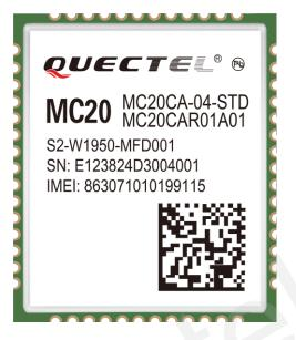
Figure 45: Top View of the Module
