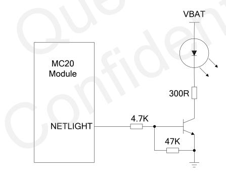
Figure 36: Reference Design for NETLIGHT
