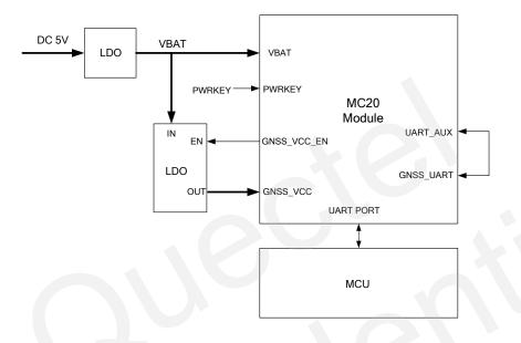
Figure 3: All-in-one Solution Schematic Diagram
