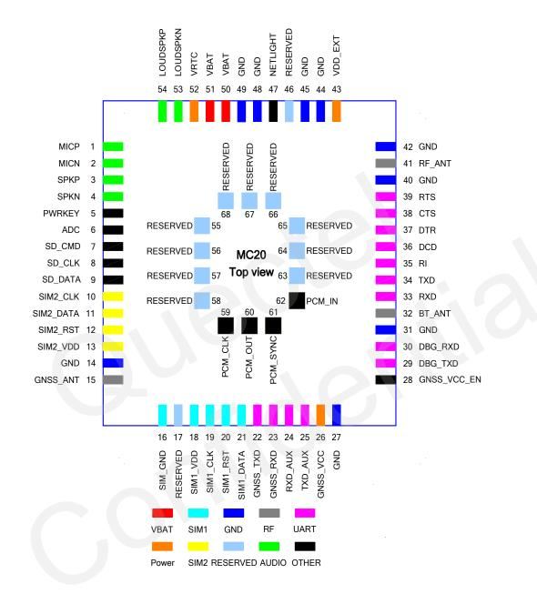
Figure 2: Pin Assignment
