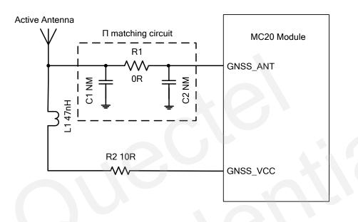
Figure 39: Reference Design with Active Antenna
