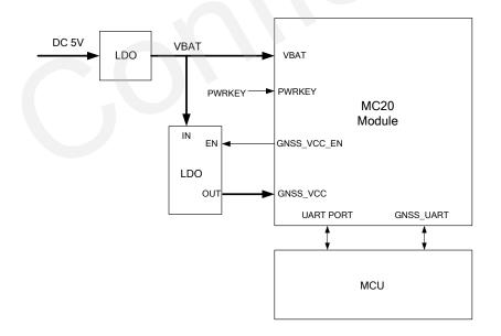
Figure 4: Stand-alone Solution Schematic Diagram
