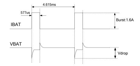
Figure 5: Voltage Ripple during Transmitting (GSM Part)
