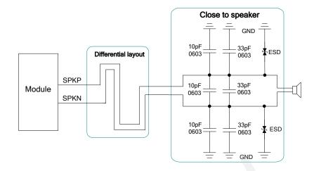
Figure 26: Handset Interface Design for AOUT1
