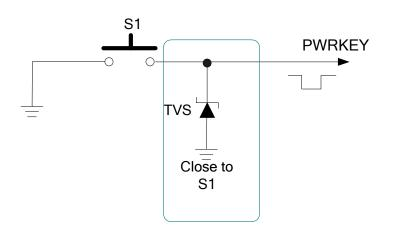
Figure 12: Turn on the Module with a Button
