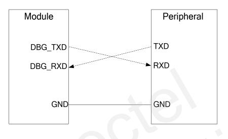
Figure 20: Reference Design for Debug Port
