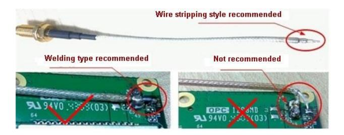
Figure 38: RF Soldering Sample
