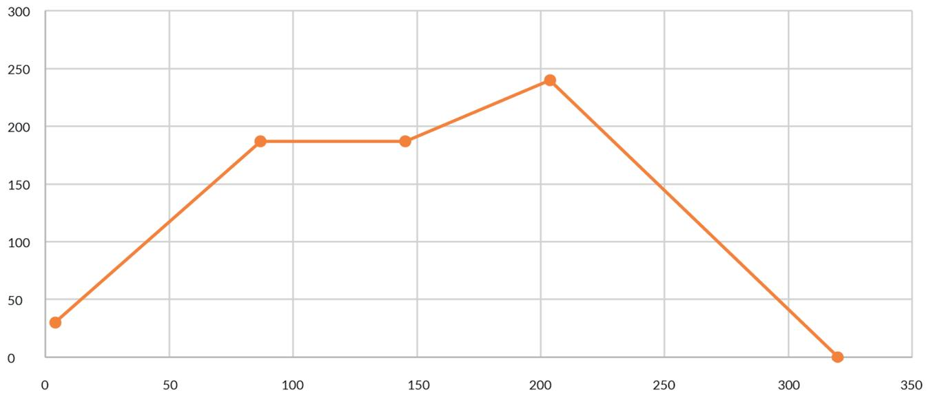
Figure 9 – Reflow soldering temperature profile (surface mount)
