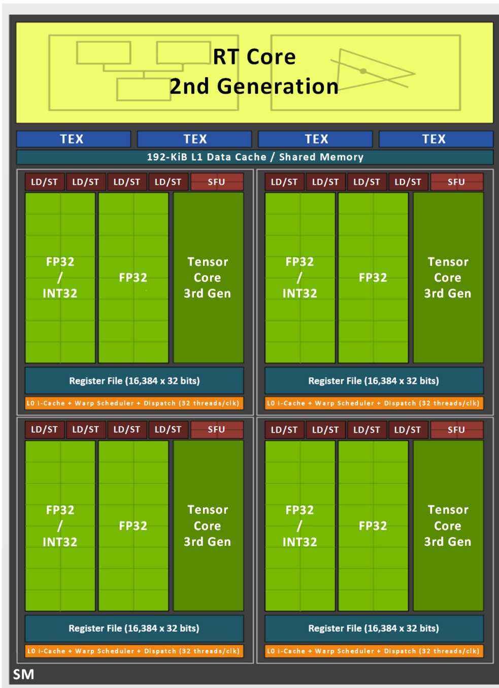
Figure 6.2 Ampere Streaming Multiprocessor (SM)
