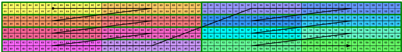
Figure 7.55 Block Linear (GPU 16Bx2 kind with TEGRA_RAW Sector Ordering).
