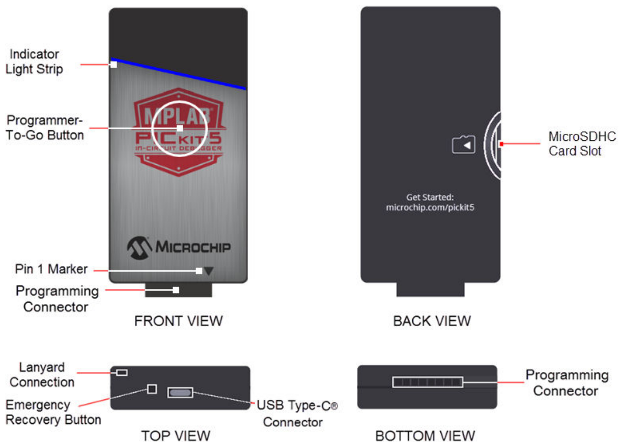
Figure 5-1. MPLAB® PICKit™ 5 In-Circuit Debugger Diagram
