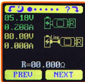
Data Connection Cable Impedance Measurement Interface
