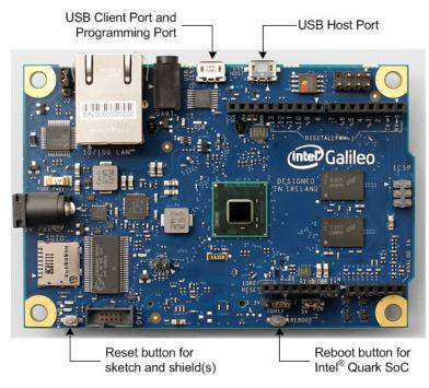
*Note:* The I/O headers are identical to the Arduino Revision 1.0 pinout.
