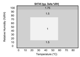
Figure 7: Typical RH accuracy tolerance over humidity and temperature for SHT45.
