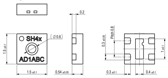
Figure 12 Dimensional drawing of SHT4x including package tolerances (units mm).
