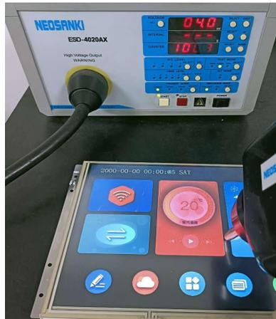
3.1 Electrostatic discharge test
