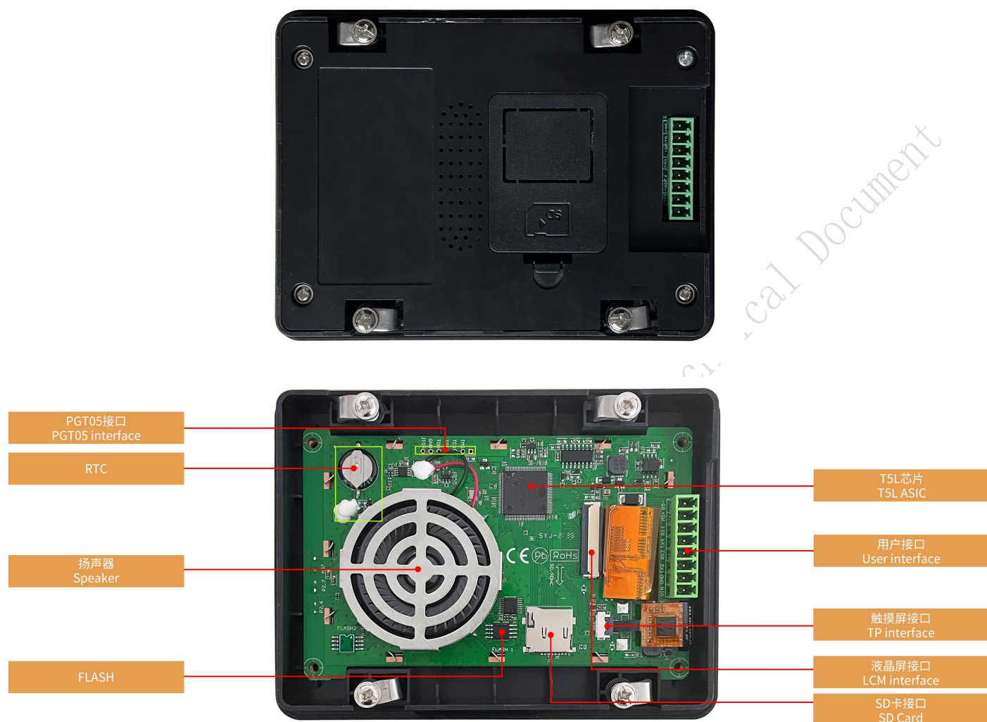
硬件接口图 Hardware interface
