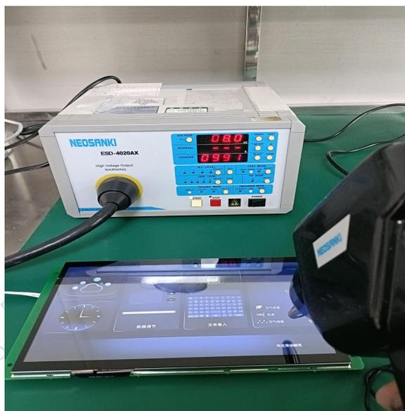
Electrostatic discharge test
