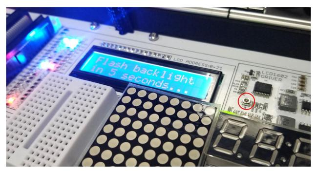
By using a standard Philips screwdriver, rotate the screw to the right or to the left when running the LCD example script in order to find the suitable brightness for you.
