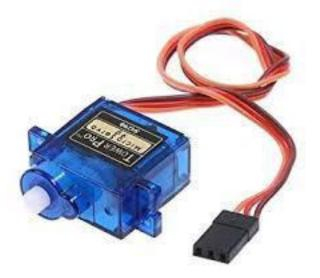
Servo is a really cool module that lets us mechanically control devices and move parts. Using this servo we can make a smart trash bin, a candy box with smart opening / closing door, and many other interesting projects!
