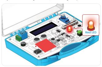
• When the light sensor is exposed to light, the LED turns off.
