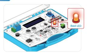
Once the program runs successfully, you will see the LED on the All-in-one Starter Kit for Arduino blinking—turning on for one second and then off for one second in a continuous loop.
