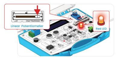
As the potentiometer slider moves, the brightness of the LED changes accordingly. When you slide it all the way to the right (maximum position), the LED reaches its brightest state; when you slide it all the way to the left (minimum position), the LED turns off.
