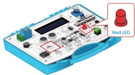
When the ambient light is dim or the photoresistor sensor is covered, the LED is initially off by default.
