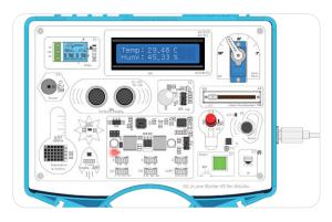
Once the program runs successfully, you will observe that the temperature and humidity values from the sensor are periodically updated and displayed on the LCD screen.
