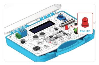
After running successfully, you will see the LED turn on when you cover the top of the light sensor to simulate low-light conditions. When you remove your hand to simulate a well-lit environment, the LED will turn off.
