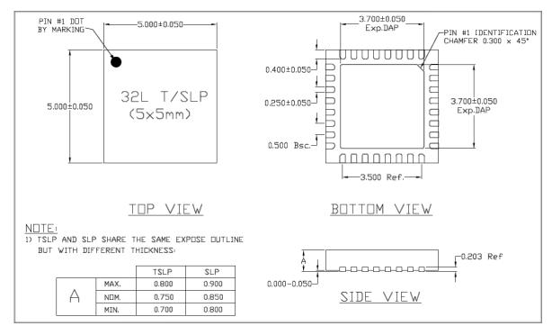
Figure 6-1. ESP8266EX Package
